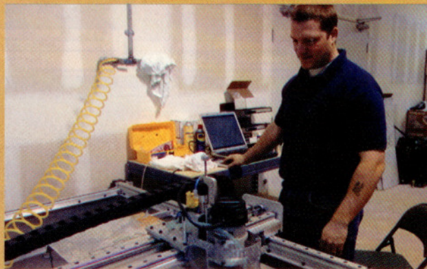
Howard Aviation's avionics shop supervisor Brian Peoples is shown overseeing the company's Panel Pro CNC milling machine as it cuts a new instrument panel. Cutouts for the Sigma-Tek artificial horizon, the altimeter, the tachometer, and one of the 6.25-by-5-inch integrated display units have already been cut.
